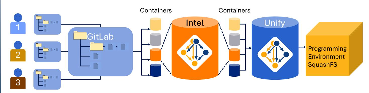
Programming environment contributors push their environment changes to GitLab, which kicks off a series of containerized CI jobs to build individual elements of the environment. The environment is then collected into a single build and compressed into a SquashFS file, which can then be distributed to the relevant machines and installed.
