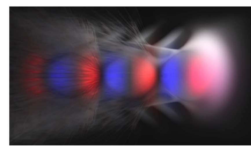
FIG. 1. Cloud render of plasma wakefield from a 3D simulation where blue (red) represents positive (negative) electric field. White represents plasma charge density.
